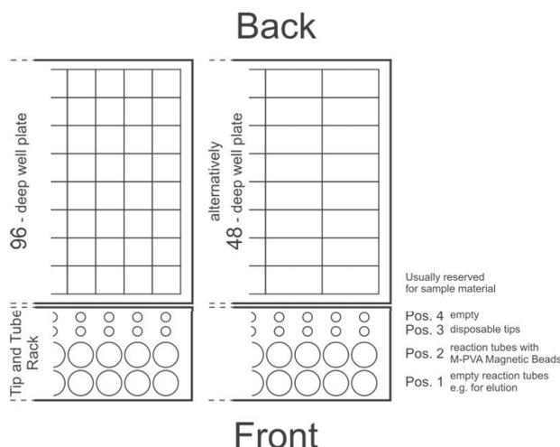
Fig. 5 Orientation of the deep well plate and Tip & Tube Rack
