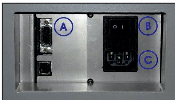
Fig. 2 Connector Terminal on the Backside of the Instrument.
